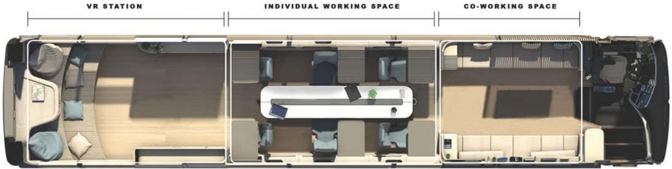
VR Station - Projector, Screen, Storages including refrigerator    Individual Work Space - Foldable Table, Rotating Seat and Hidden Table    Co-Working Space - TV, Sofa, Wall Panel
